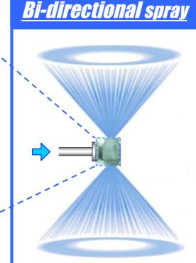
The TWAA series is **<u>bi-directional</u>**, so one nozzle unit can take the place of two.
