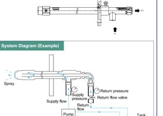
Steam-driven nozzles, JOKIJet<sub>®</sub> series, uses steam instead of compressed air to atomize liquid. Please inquire with us for details.
