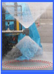
With 2 orifices, the flow normally sent through 1 orifice is halved, yielding smaller droplets. Best for applications with contact / reactions.
