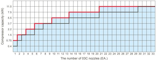
Notes: 1. When spraying at 0.3 MPa air pressure, please refer to the black line ( — ). When spraying at 0.5 MPa air pressure, please refer to the red line ( — ).
