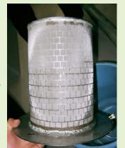
After 30 seconds\* of high-pressure jet cleaning, the filter has been cleaned. \*The cleaning time depends on unfiltered water conditions.
