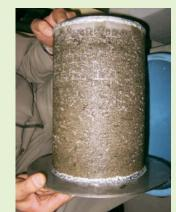
Foreign particles thickly-sedimented on the filter.
